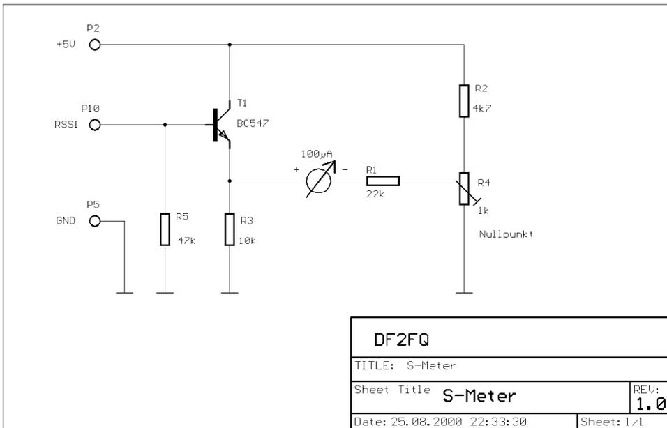
Fig. 6, example for a simple S-meter circuit
