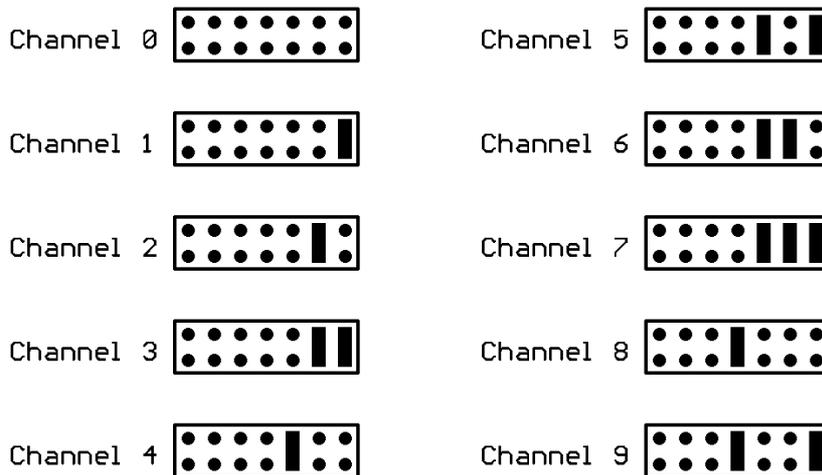
In the original configuration the 10 channels are pre-programmed with 430, 431,... to 439 MHz. Programming of the desired frequencies is done through the serial interface. You need a computer with a RS232 interface (e.g. COM1 or COM2 at DOS computers) and any V24-terminal software which is capable to send characters to it. Such a software is part of most operating systems. Depending on the connector type please regard to table 3 for the exact configuration.
